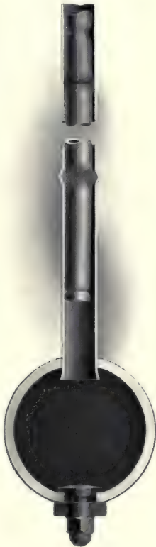
CROSS SECTION SUPER-HEATER HEADER SHOWING HANDHOLE FITTINGS ASSEMBLED AND METHOD OF HOLDING CORE IN PLACE
